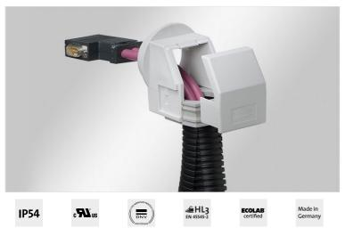
The split KVT-W90 cable glands are used to insert and seal pre-terminated cables at a 90° angle. But also electric, pneumatic or hydraulic lines without terminals or connectors as well as corrugated conduits can be easily routed (e.g. into control panels, enclosures or machinery) and sealed with IP54.
